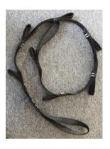
Set breaking load – 50 kN Test data: 19.09.2019
